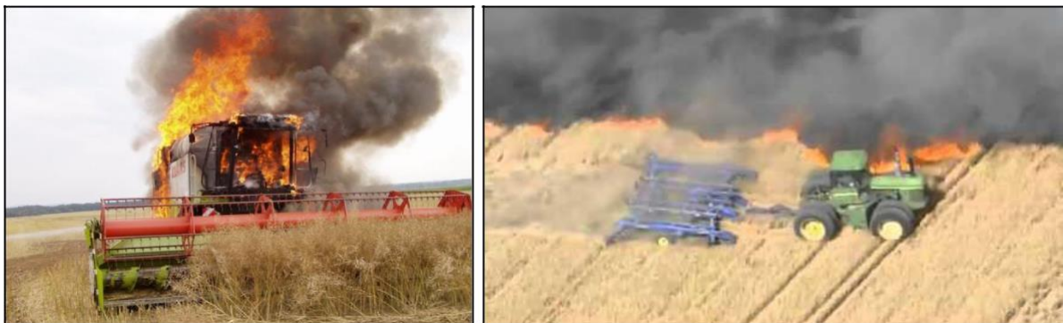
Figure 3 Fire of a grain harvester in the rape of oilseed rape (Černek, 2015 ww.sme.sk) and mitigating the spread of fire with shallow tillage tools (www.youtube.com)
