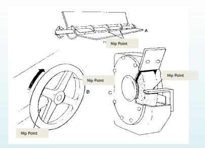
Nip points can occur between rotating and stationary parts, which produce a shearing, squeezing or grinding effect.
